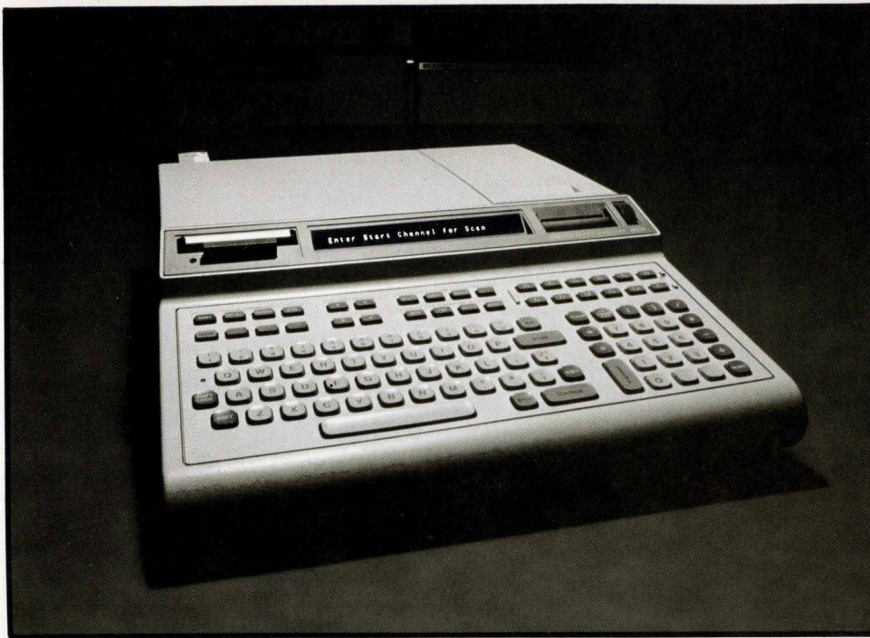
Fig. 5. Model 9825A Calculator was the first product to use the new HDSP-2000 display. The calculator's display is controlled by a dedicated custom LSI chip shared with the calculator's printer. The calculator's processor feeds the characters to a ROM in the custom LSI chip, and the chip's circuits then process the character data for display. The 32-character display has a refresh rate of 128/s and a duty factor of 17%.
